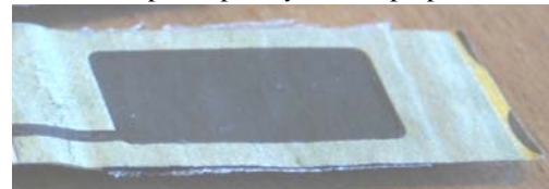
Figure 1. Sensor element consisting of two layers of “newspaper grade” paper with zinc based ink (top layer) and carbon based ink (bottom layer). Absorbing layer (doped with electrolyte and dried) is placed in between the active layers.
